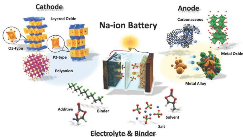
**Figure 1.** Different electrode structures in sodium-ion batteries (Picture credit: Creative Commons)
