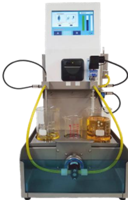
Figure 2. Representative filter-blocking-tendency apparatus used for controlled filtration tests.
