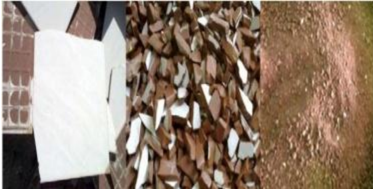
Figure 2. Crushed ceramic tile processed for use as fine-aggregate replacement.
