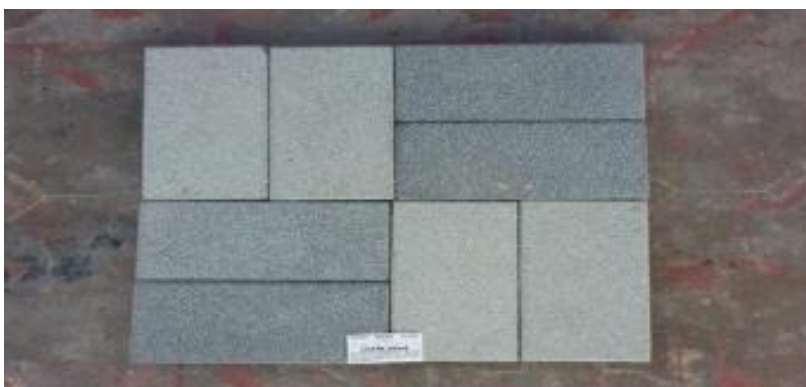
Figure 1. Representative conventional concrete utility block used as the reference specimen.
