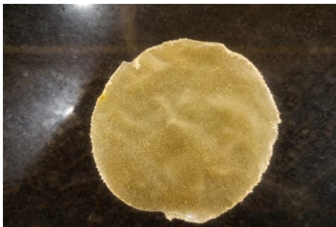
Figure 2. Representative chitosan/gelatin/starch film containing muskmelon peel extract prepared by solution casting.
